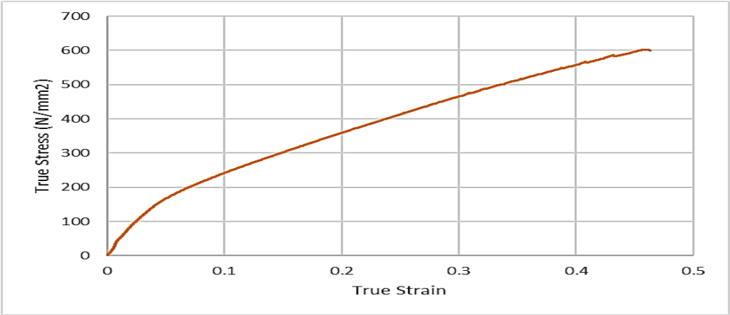
Fig. 3. True stress and True strain curve for brass alloy
