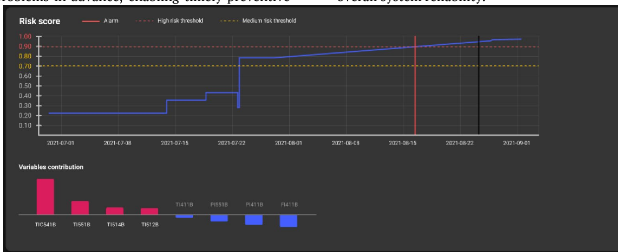
Fig. 6. Using sensor data for anomaly detection and equipment failure prediction
