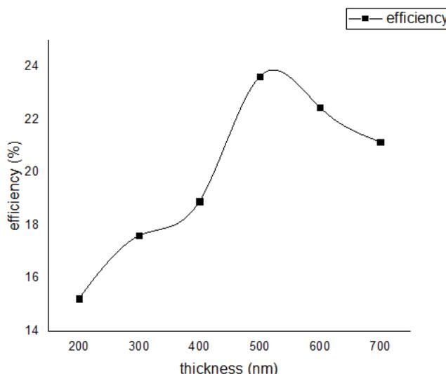
Fig. 3. The efficiency of the structure in different thickness of pervoskite layers
