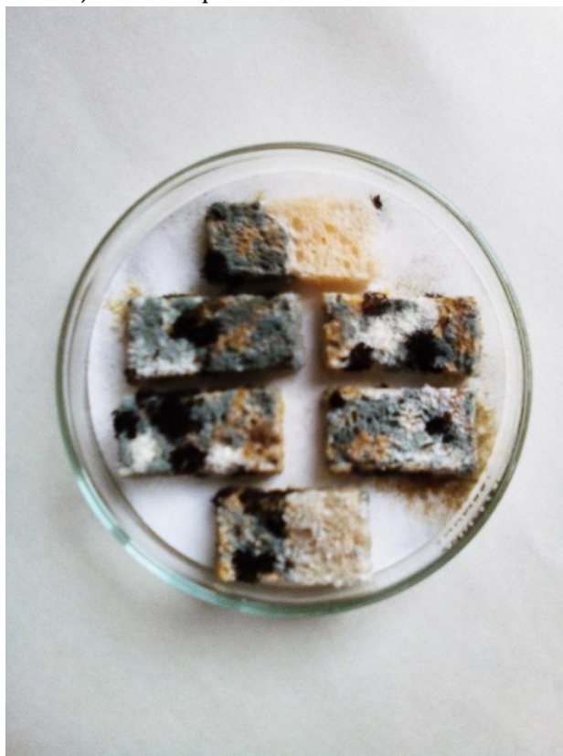
Fig. 4. Antifungal activity of CuL_2 against bread mold ( Mucor mucedo ) after exposure in a chamber with saturated water vapor for 5 days at 298 K. Four central samples were untreated with catalysts
