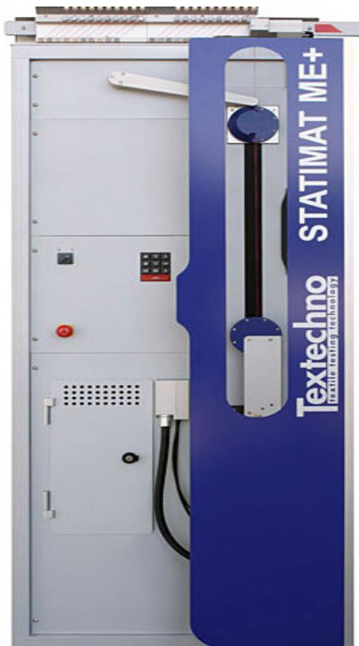
Fig. 4. The STATIMAT ME breaking machine
